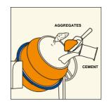
Add one heaping scoopful of MasterLife CH 500 per bag of cement consumed and dry mix with cementitious binder, sand and coarse aggregates
