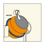
Add the required water into the mixer as per the water cement ratio and mix judiciously. Add MasterPel 777 (Optional)
