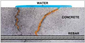
When treated with MasterLife CH 500, the specialized polymers lie dormant within the pores and capillaries of concrete and are activated on contact with ingressed water. What follows is a chemical reaction resulting in the formation of non-soluble gel that plugs and heals the crack in concrete over time.
