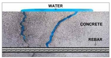
Microcracks occurring in concrete allow the ingress and passage of water, chlorides and other harmful substances that lead to corrosion of reinforcement and damage to the structure.
